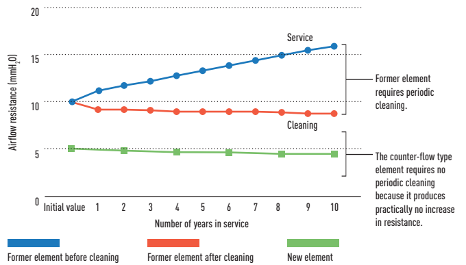
Changes in airflow resistance based on number of years in service.
